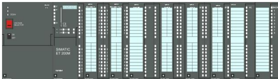
Figure 6: remote I/O ET200M rack
